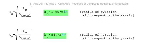
K. CALCULATE THE RADII OF GYRATION OF THE COMPOSITE AREA WITH RESPECT TO THE CENTROIDAL AXES
