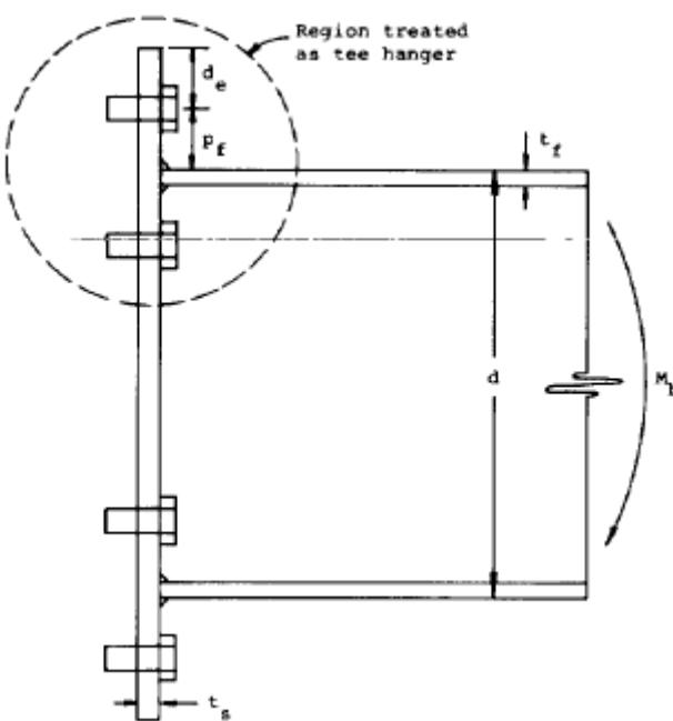
Maximum bending moment for maximum bending stress of 0.66 \$F\_y\$,
