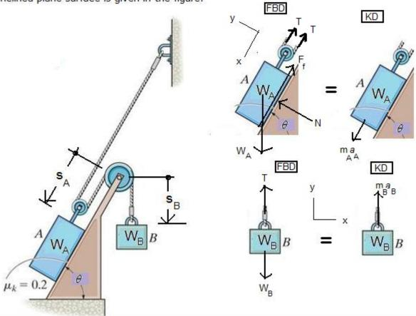
Kinematics of the two blocks (absolute dependent motion):  $2 \cdot s_A + s_B = L$
